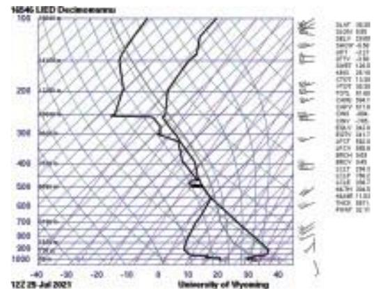
Figure 10. Atmospheric radiosonde at Decimomannu (CA) at 2.00 p.m. on 25 July 2021. A significant saturation deficit is still evident, especially below 3000 m or 700 hPa. In addition, there is an imposing layer of near saturation air above 4000 m altitude.
