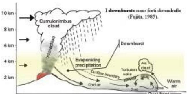
Figure 8. Simplified diagram of the interaction between the smoke plume and a storm cell. Water droplets that form at high altitudes by condensation of atmospheric vapour precipitate downwards. However, upon encountering a layer of very dry and warm air, they evaporate, cooling the air and creating strong downdrafts that reach the ground and propagate in all directions (adapted by Cabiddu from Knippertz et al., 2007).
